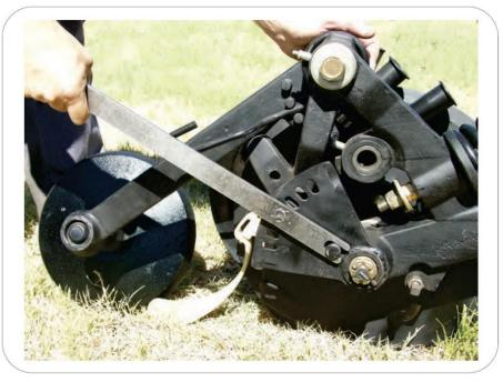
A special tool for displacing a punched plaque in one way or the other is used to adjust levelling wheel position.
