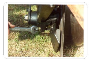
The drop bolt (2) must let the shoe swing freely (2.5cm) so that a self-cleaning action can take place. If it is too tight against the shoe the spring will not work and the set will wear faster or break as blockage will be produced. An advantage of tight fitting is the possibility of working on damp soils.
