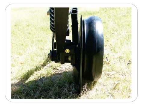
The 3mm opening between the lip of the tyre and the coulter is aimed at reducing tyre wear. It is adjusted by means of steel washers and it allows the wheel to come into slight contact with the disc when the drill is at work
